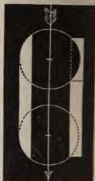
FIG. 161.—The Construction of a Convex and a Concave Cylindrical Lens from a Cylinder.
